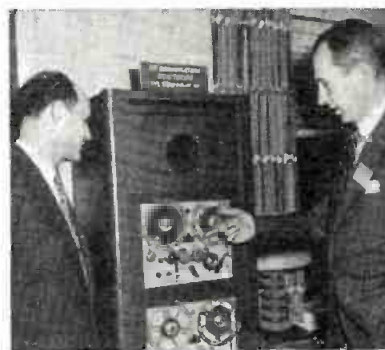
TAPE RECORDER which passes tape one inch per second was shown in the suite of Presto Recording Corp., as demonstrated by John Strampfer (l) and Tom Aldrich.
